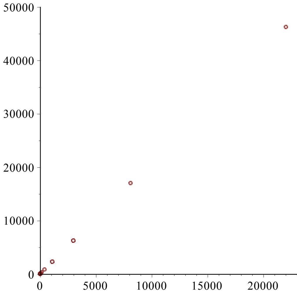
These points (plotting  $y$  versus  $e^x$ ) look like a straight line through the origin, so we conclude that the data does support  $y$  being proportional to  $e^x$ .
